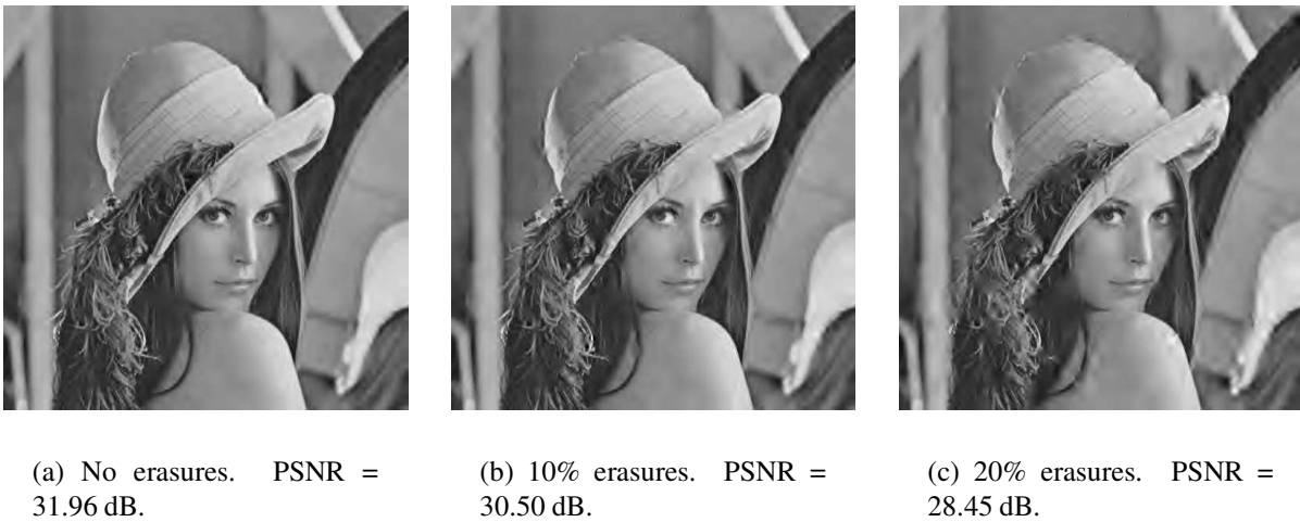
Figure 5.6 Example decoded images for multistage PZW under three erasure conditions.
