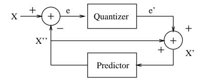
Figure 1.1. Differential Pulse Code Modulation
