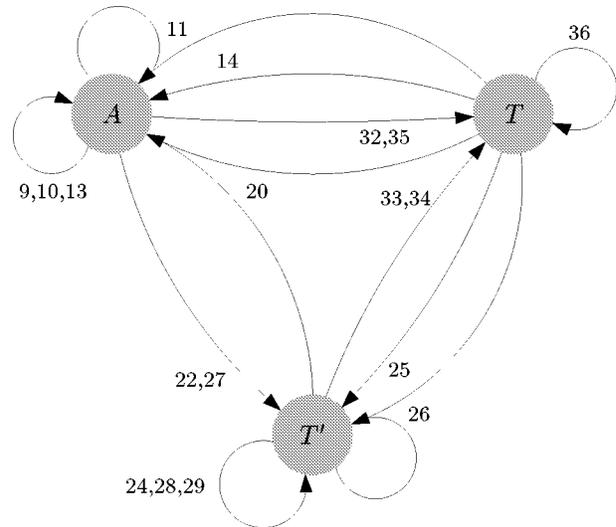
Fig. 1. The interdependence between bounds on the three types of binary constant-weight codes:  $A$  stands for general constant-weight codes,  $T'$  for doubly-bounded-weight codes, and  $T$  for doubly-constant-weight codes. Numbers refer to theorems in this paper. For example, the arrowhead labeled 20 represents a bound on  $A(n, d, w)$ , derived in Theorem 20, in terms of bounds on doubly-constant-weight codes and bounds on doubly-bounded-weight codes.
