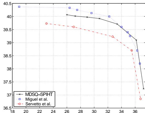
8, and we compare MDSQ-SPIHT with the scheme of Miguel *et al.* [9], and with the ULP scheme of Mohr *et al.* [11]. Using 5 diagonals, our coder performs close to their schemes when there is no description loss, but is about 3 to 5 dB worse than that of [11] when there is a loss of 1 to 2 descriptions; on the other hand, MDSQ-SPIHT performs better than [11] when at least 4 descriptions are lost, and the gain is as high as 10 dB when only 1 description is received.
