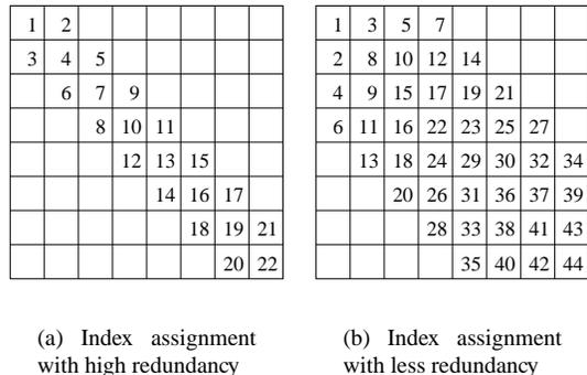
**Fig. 2.** Example MD index assignment mappings for two descriptions.
