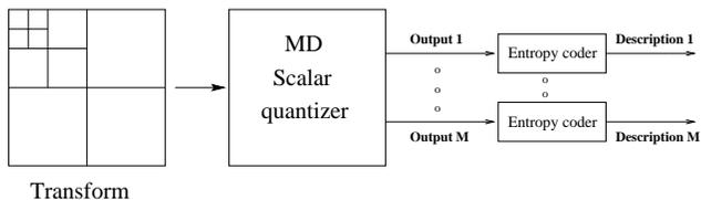
**Fig. 1.** Block diagram of an image coder for packet loss channels.
