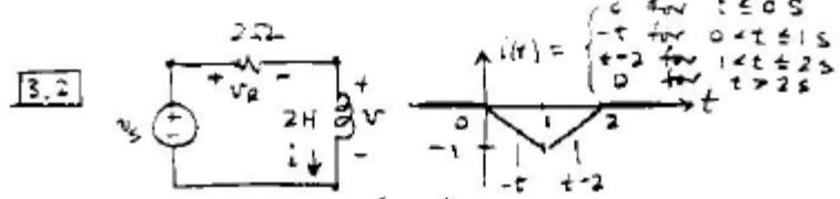
(a)  $v_R(t) = L \frac{di(t)}{dt} = 2 \frac{di(t)}{dt} = \begin{cases} 0 & \text{for } t \leq 0 \\ -2 & \text{for } 0 < t \leq 1 \\ 2 & \text{for } 1 < t \leq 2 \\ 0 & \text{for } t > 2 \end{cases}$
