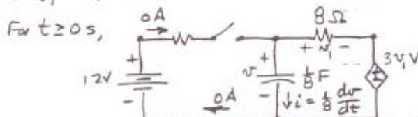
$$\text{By KVL, } v - 3v_1 - v_1 = 0 \quad \text{By Ohm's law, } v_1 = -8i$$
