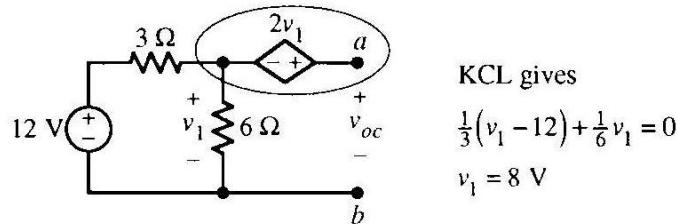
KVL gives  $v_{oc} = 2v_1 + v_1 = 3v_1 = 3(8) = 24 \text{ V}$
