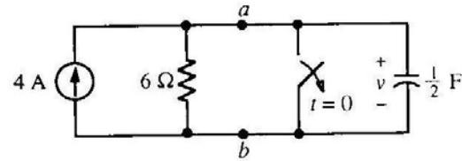
With the switch closed, we obviously have  $v(0^-) = 0 \text{ V}$  so  $v(0^+) = 0 \text{ V}$
