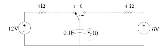
(b) Suppose the switch, after having moved over to the right at t=0, were to go back to the left at t=0.2s. Find an expression for the voltage across the capacitor,  $V_C(t)$ , for t>0.2s.
