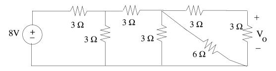
Problem 2: Find  $I_o$  in the following circuit using linearity and the assumption that  $I_o = 1$ A.
