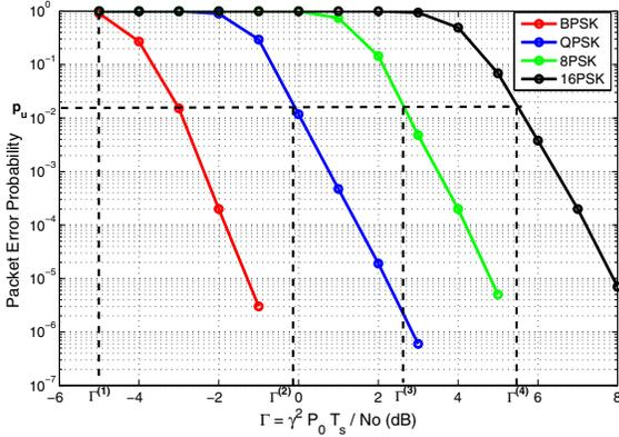
Fig. 2: Packet error rate vs. instantaneous received SNR.
