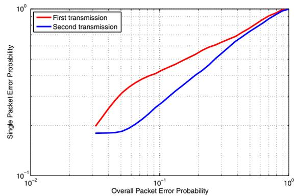
Fig. 5: Single transmission PER for the two transmissions.
