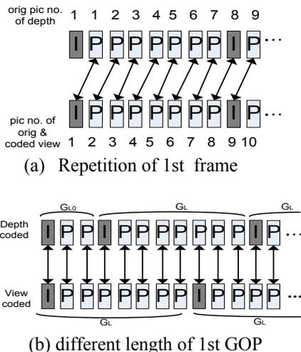
Fig. 2.1 Alignment of view and depth sequence
