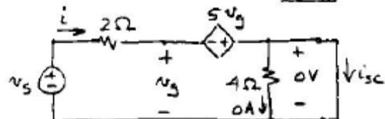
$$\text{By KVL, } v_s = 2i - 5v_g \quad \text{Also, } -v_g - 5v_g = 0$$
