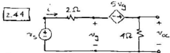
$$\text{By KVL, } v_s = 2i - 5v_g + 4i \quad \text{Also, } -v_g - 5v_g + 4i = 0$$
