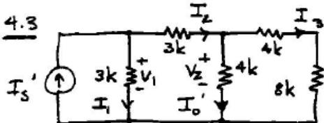
$$I_3 = 2 \text{ mA} \quad I_0' = 1 \text{ mA}$$
