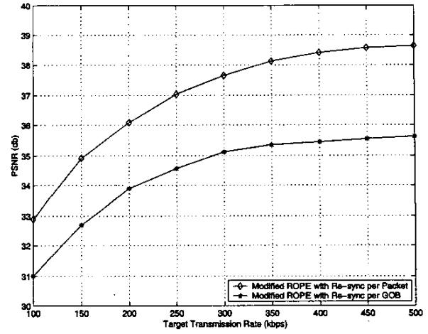
Fig. 5. PSNR performance versus transmission rate. "Salesman" QCIF sequence at 10fps, packet erasure rate  $p=5\%$ , bit error rate  $Pb=0.01$ , and fixed-packet length 800.
