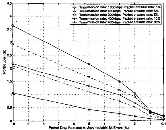
Fig. 2. PSNR loss over different target packet drop rates. "Carphone" QCIF sequence at 10fps and fixed-packet length 400.
