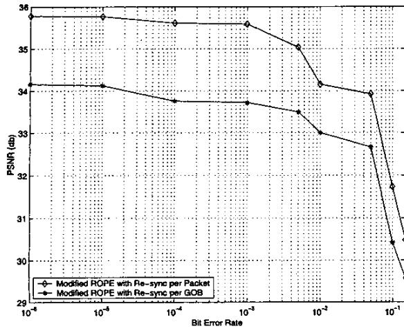
Fig. 4. PSNR performance versus bit error rate. "Container" QCIF sequence at 15fps and 150kps, packet erasure rate  $p=5\%$  and fixed-packet length 400.
