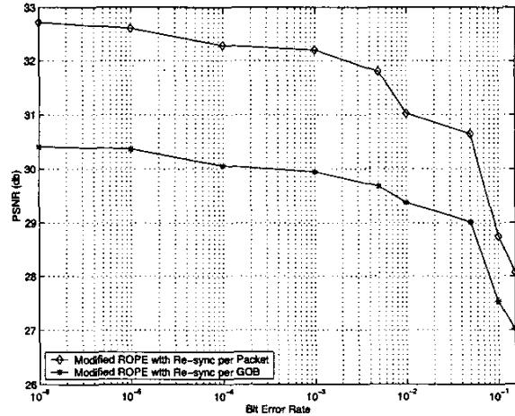
Fig. 3. PSNR performance versus bit error rate. "Carphone" QCIF sequence at 30fps and 400kbps, packet erasure rate  $p=10\%$  and fixed-packet length 400.
