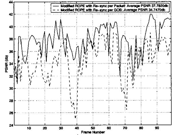
Fig. 6. PSNR performance versus frame number. "Salesman" QCIF sequence at 300kbps and 10fps, packet erasure rate  $p=5\%$ , bit error rate  $Pb=0.01$ , and fixed-packet length 800.
