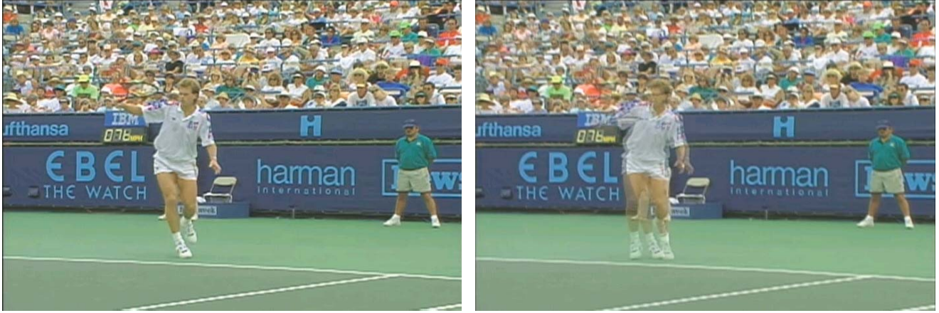
(a) Lost frame number 35 of Stefan. Whole frame concealment by JM decoder with frame copy. (b) Lost frame number 35 of Stefan. Whole frame concealment by FFMPEG decoder with temporal frame interpolation.
